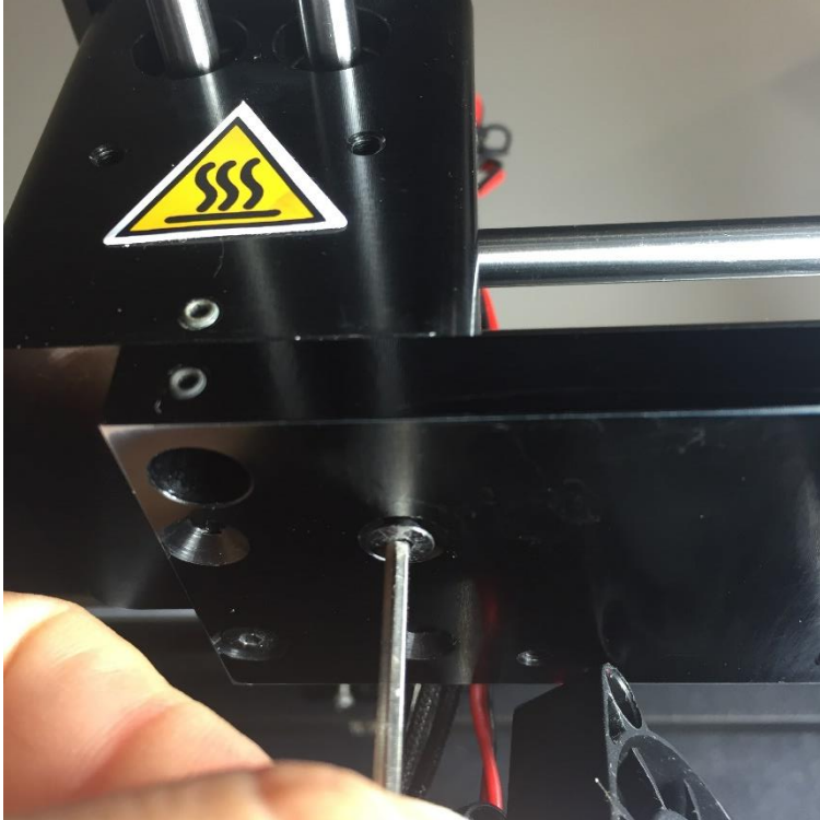
10. Remove cooling block using 2.0mm Allen Key.
