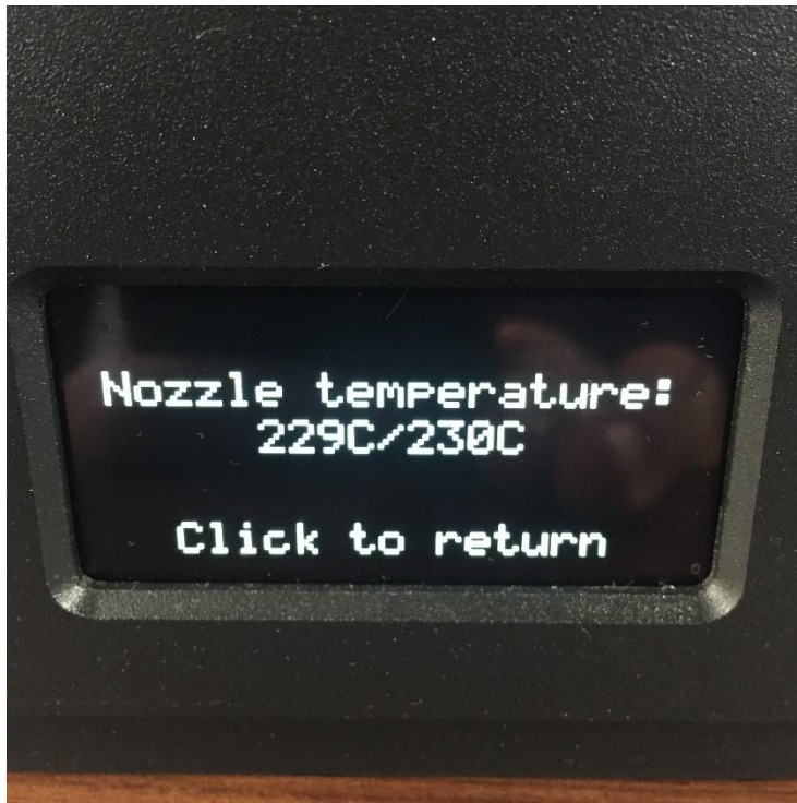
18. Preheat the nozzle to 230C.
